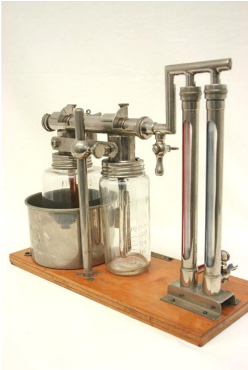
VGKM0541 – Anaesthesia apparatus (combined flowmeter/rotameter, manifold, chloroform and ether vaporisers), mfr. A. Charles King Ltd. (England).
